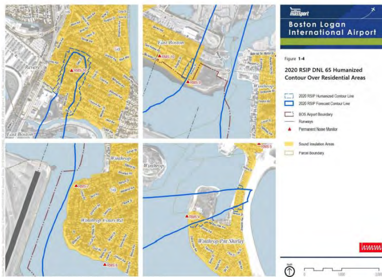
Figure 5.4-6 65 DNL noise contours adjusted for land use
