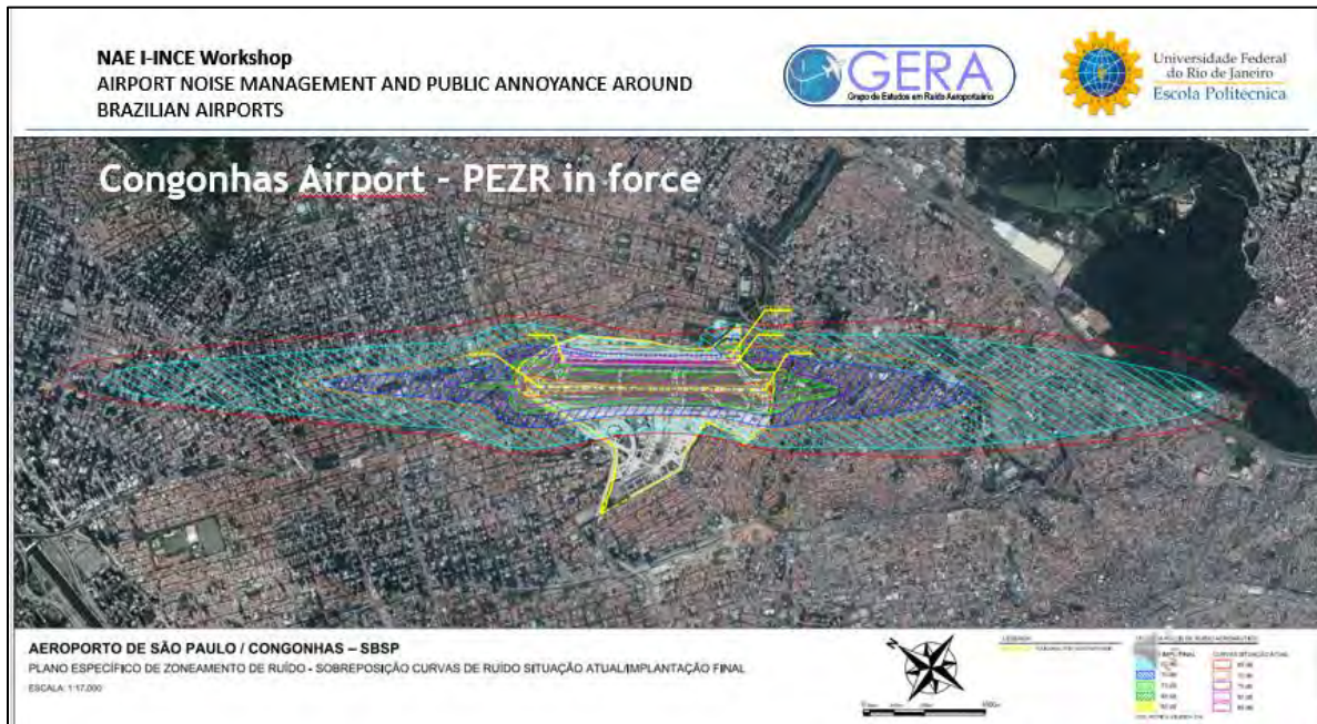
Figure 5.3-3 Research into airport noise levels: Example of noise contours at Congonhas Airport
