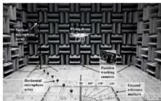
Figure 8.2-4 Noise measurement of small/medium drones
