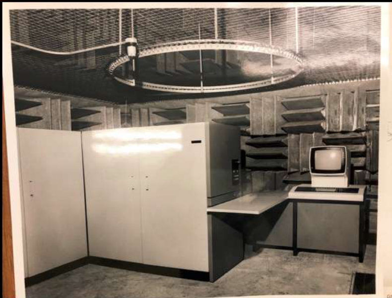
Figure 2.4-3 The fully anechoic chamber that could be converted into a hemi-anechoic chamber by Bill and laboratory staff moving the wedges
