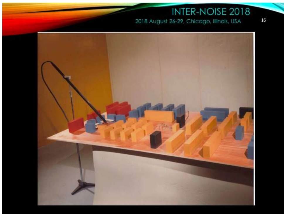
Figure 2.4-10 Example of scale modeling of a data center using a spark source and a miniature microphone (by Russ Wise)
