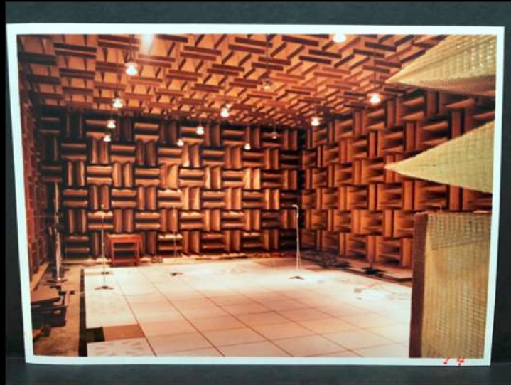
Figure 2.4-7 Large new wing with a hemi-anechoic chamber, with a special raised floor for testing a new line of mainframe computers
