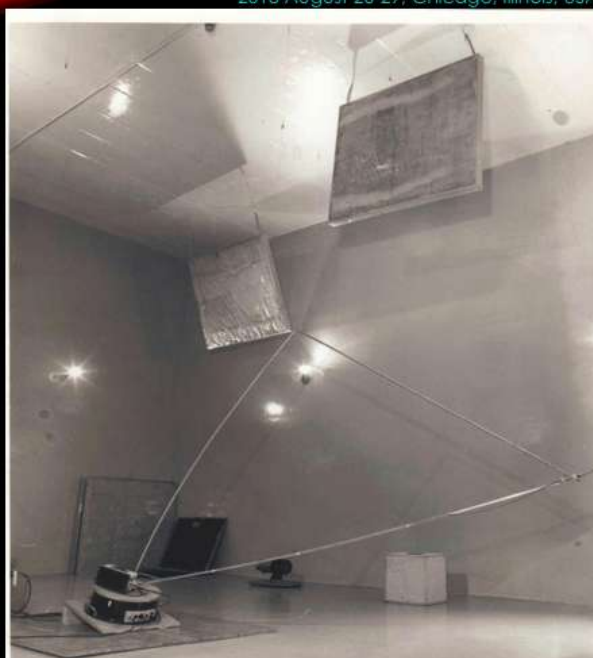
Figure 2.4-4 The reverberation room in the original building with the first rotating microphone boom constructed at IBM
